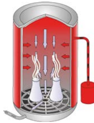
Drying vacuum with heating of the double jacket, V version
