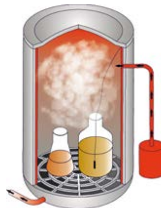
Steam generation using the built-in steam generator
